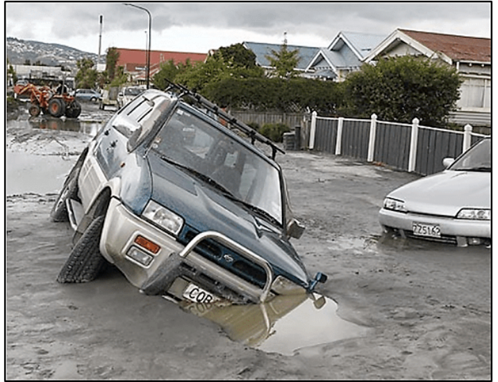
Caption: Structural damage (left) and vented sands from liquefaction (right) from the 2011 Christchurch earthquake in New Zealand.
