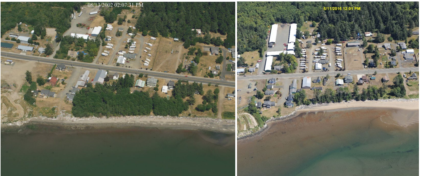
Aerial photographs of the site from 2002 (left) and 2016 (right) show shoreline trees lost to erosion. Note presence of shoreline armoring in 2016 photograph—shoreline stabilization structure was later installed on the beach to the right of this armoring. (Image credit: Washington State Department of Ecology's Coastal Atlas)
