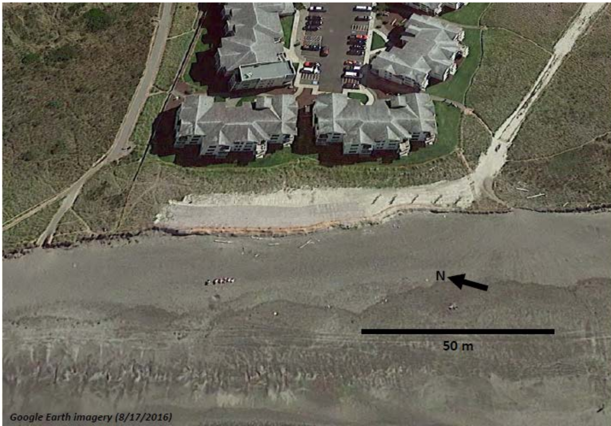
Figure 3-3: Aerial view of emergency protection measures in place in 2016 and 2017 in response to severe dune erosion episodes in 2015 / 2016
