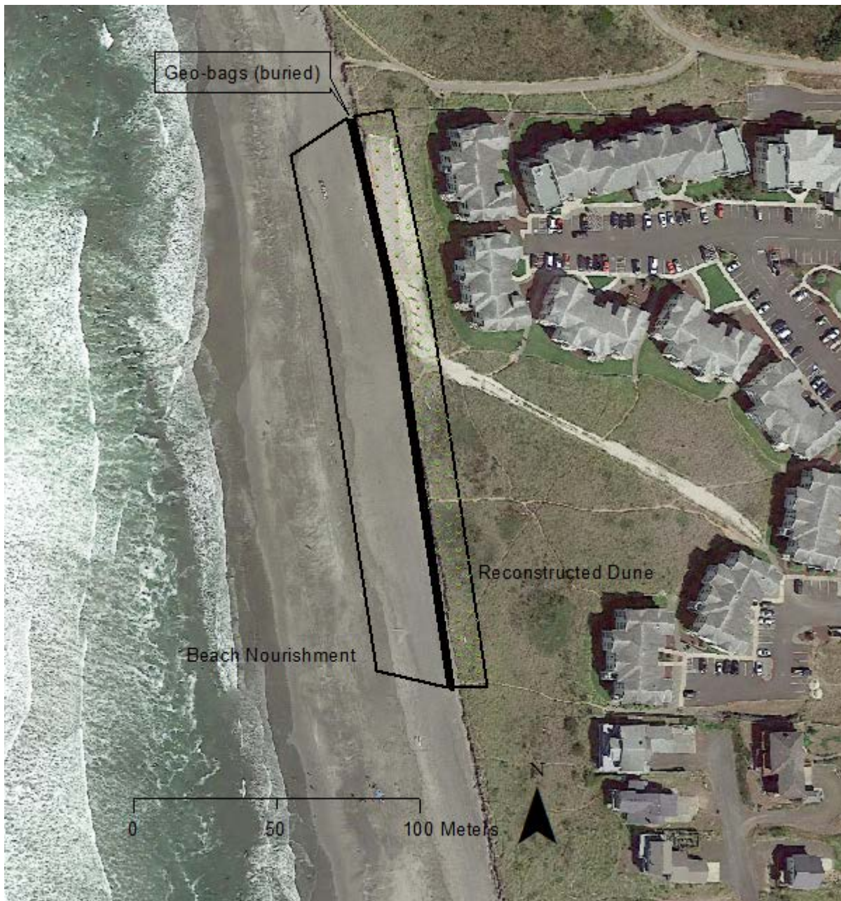
Figure 4-7: Plan View for Option 3 - Large geotextile bags (sand filled) dune core with sand beach nourishment and dune reconstruction
