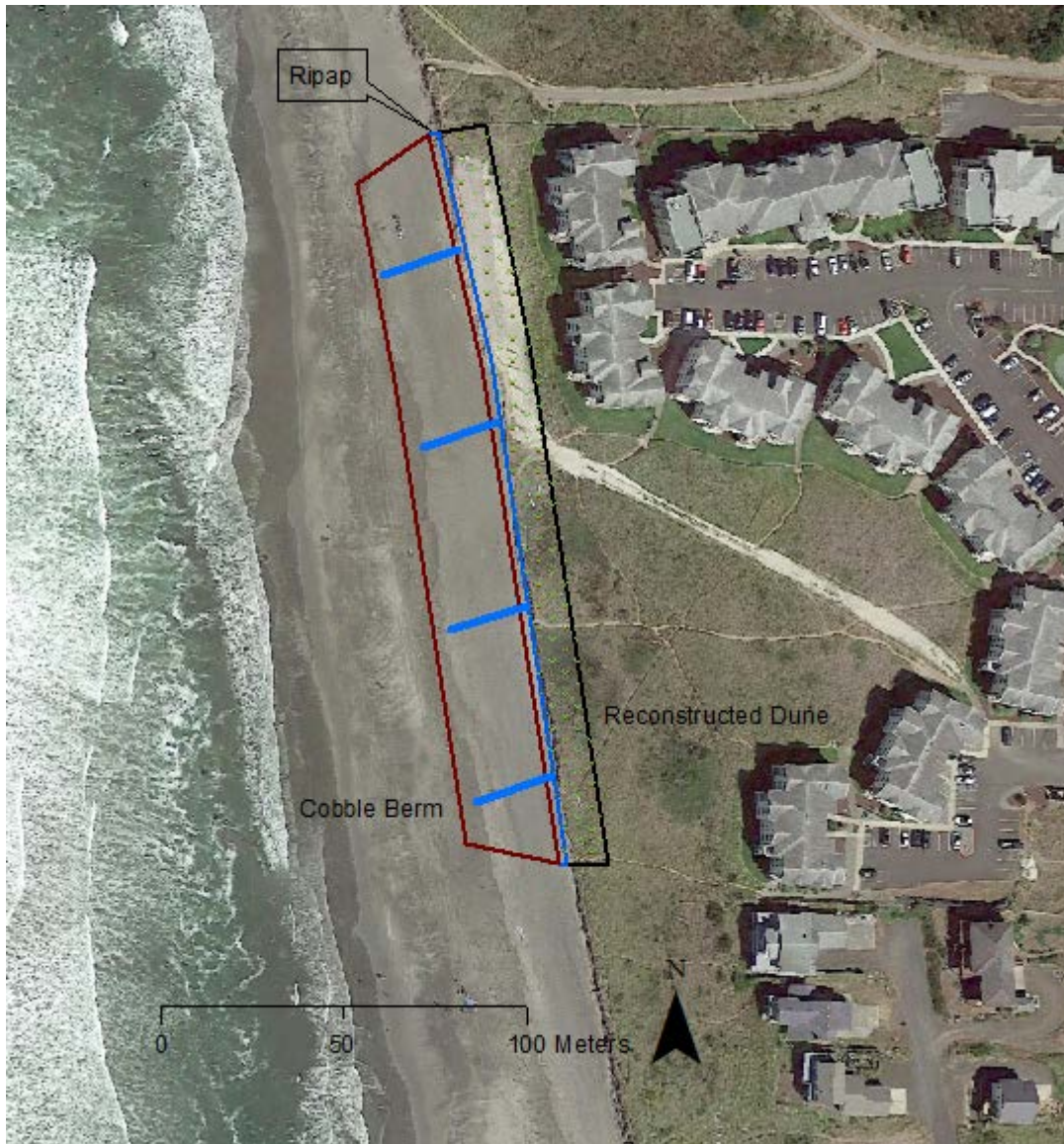
Figure 4-5: Plan View for Option 2 – Rip-rap revetment with dynamic cobble berm toe; optional finger dikes and dune reconstruction
