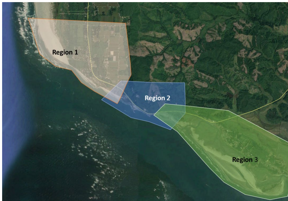
The North Cove shoreline is comprised of three distinct regions, each with differing conditions influencing erosion trends. The North Cove Dynamic Revetment addresses erosion in Region 1 and is coordinated with two other projects working in the adjacent regions. (Image credit: Washington Coastal Hazards Resilience Network )
