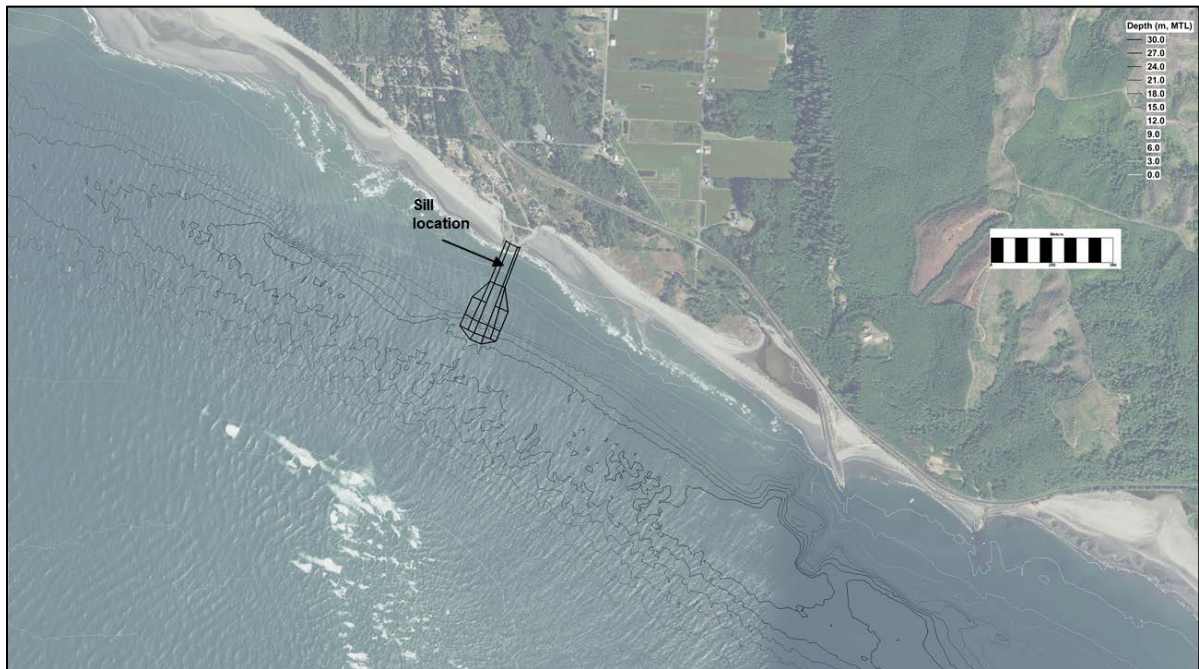
Figure 39. New Training dike - Alternative 1a without sill; Alternative 1b with sill.
