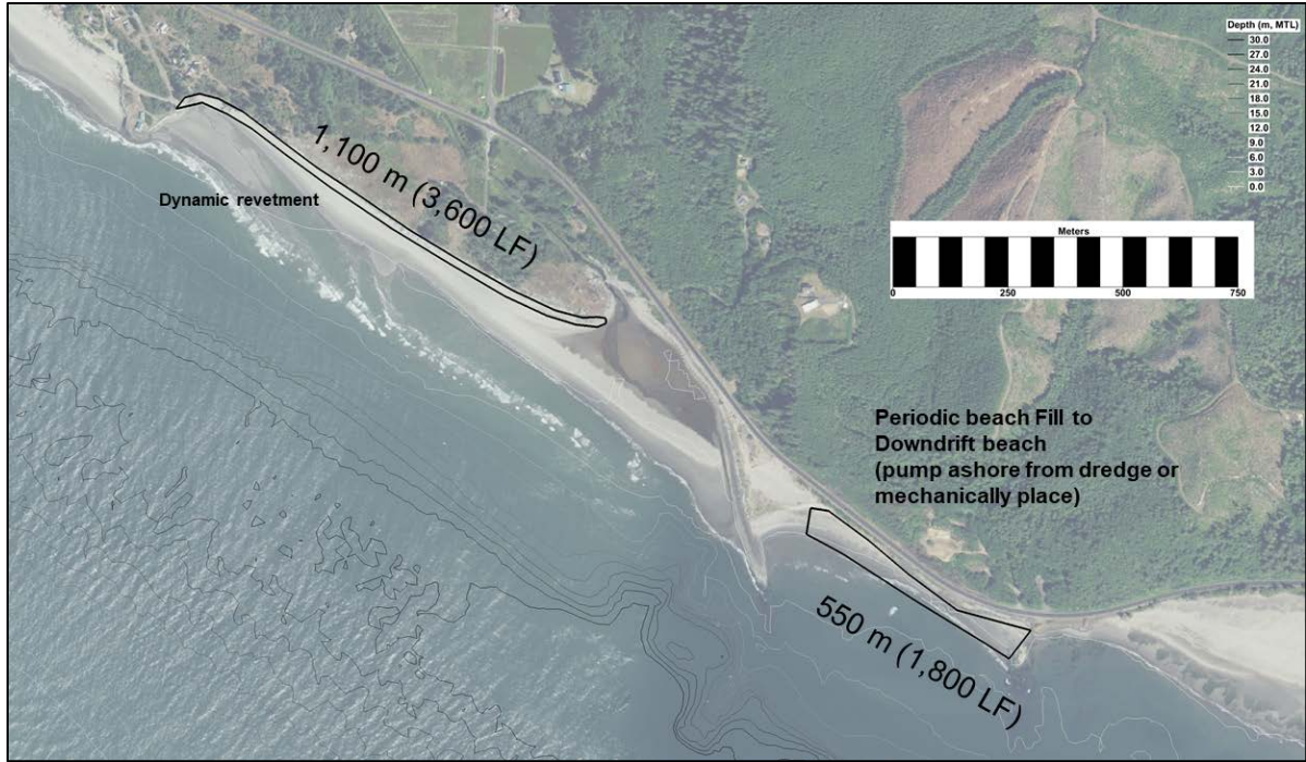
Figure 42. Alternative 2c. Dynamic revetment with beach fill
