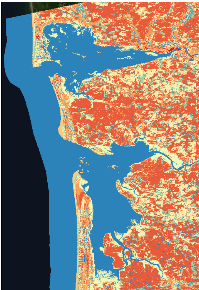
Figure 36: Preliminary Bed Friction Factors (Manning's n ) Based on the 2016 NLCD Dataset (0.02 for Open Water [Blue] to 0.15 for High-intensity Development [Red])
