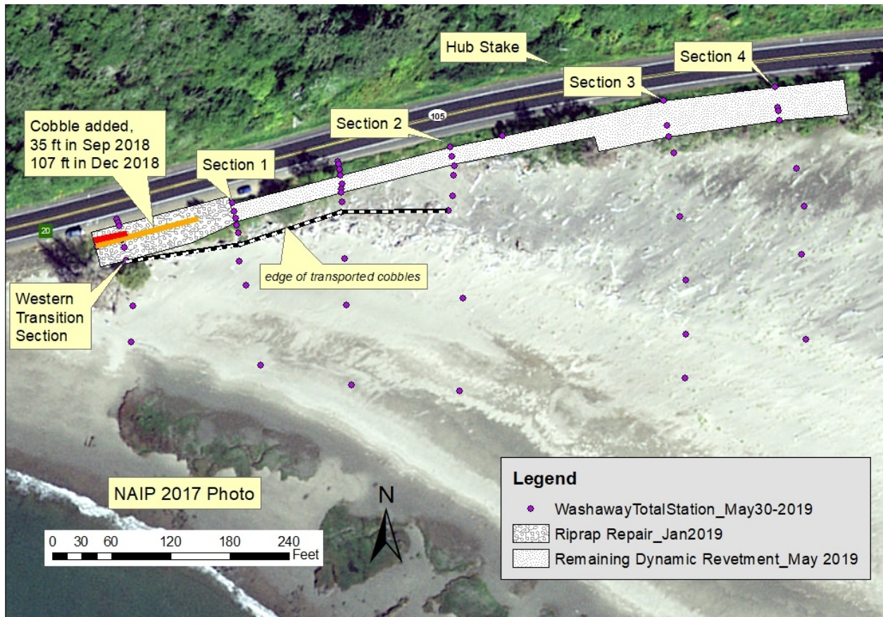
Figure 7. Map of the 2018-19 repairs and May 2019 survey.
