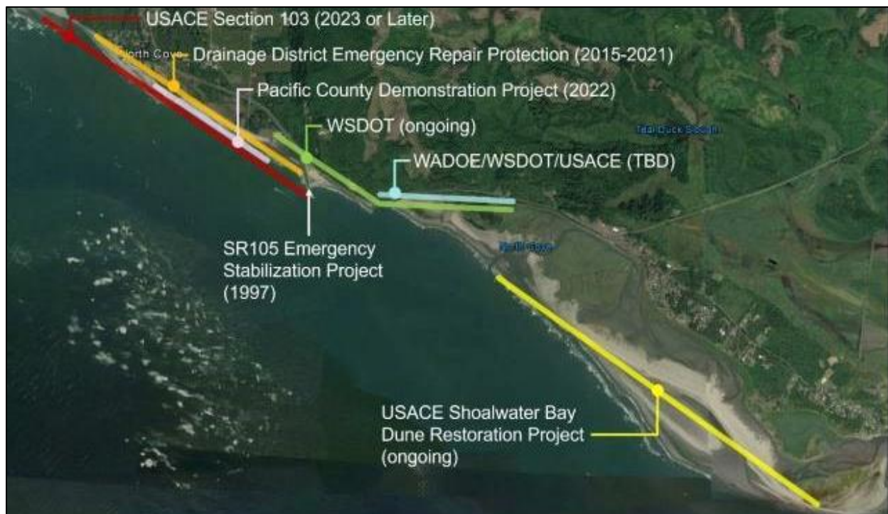
Figure 7. Ongoing and proposed erosion protection projects in the region of North Cove and Tokeland, as of January 2021. Provided by Mott MacDonald.
