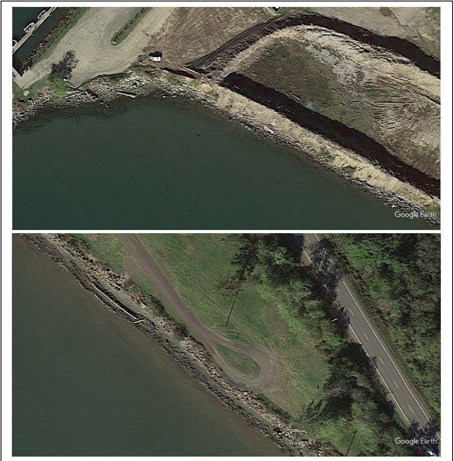
Figure A.8. Areas of erosion east of Chinook Marina (top), and at Chinook County Park one mile southeast of Chinook Marina (bottom), due to bank revetment damage from ongoing wave action. At Chinook Marina, dredge disposal activity is evident in the adjacent parking lot. Source: Google Earth 2018 image.
